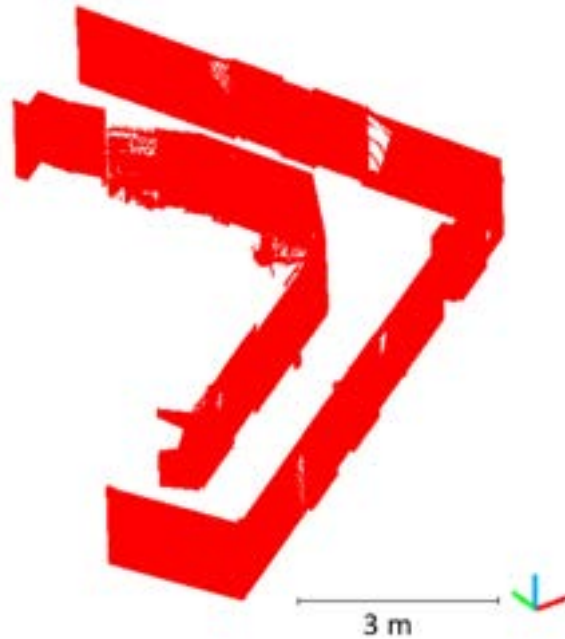
Figure 5. Slanted view of the TLS 3D point cloud for the ITC1 dataset. The ceiling and floor points are not shown for visualization purposes.
